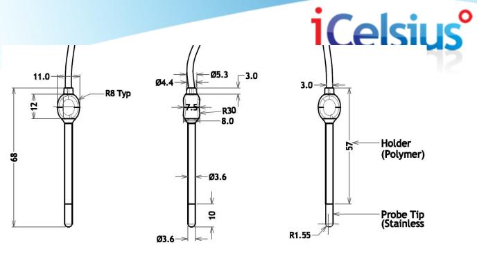
(dimensions in millimeters, connector not illustrated)
